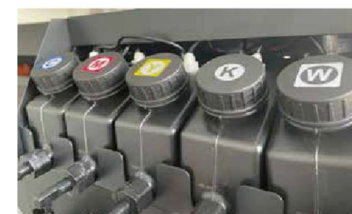
500ml large capacity ink supply system
