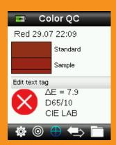
Measure samples and display Pass/Fail warnings. Save up to 350 samples with voice or text tags
