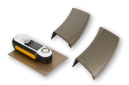
RM200QC measures color accurately by taking images of your sample using 8 different visible illuminations and 1 UV LED (9 bands), an advantage over traditional colorimeters that typically have only three 3 bands (Red, Green, and Blue).
