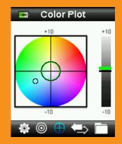
Simple to understand color plot shows the difference between standard and sample.
